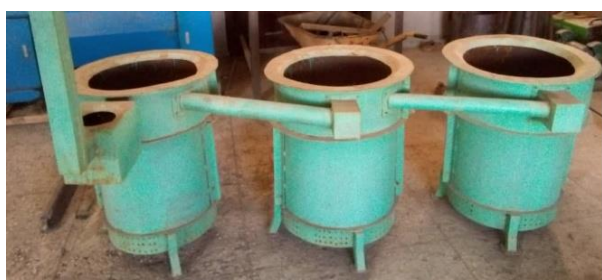
Plate 1: The Prototype Model of the Cascaded three pots stove
