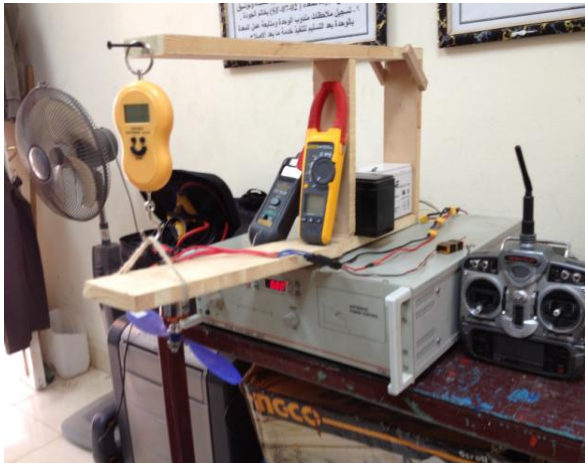
Figure 4: Motor test setup for thrust calculation.
