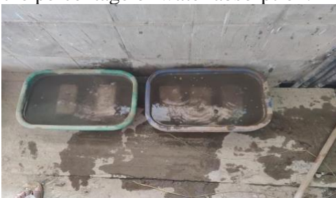
Figure 6: Water absorption test on SSA blocks.
