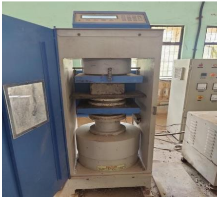
Figure 5: compressive test on SSA blocks.
