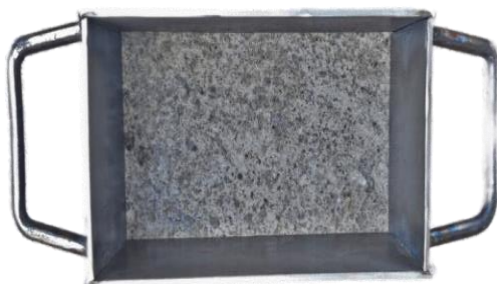
Figure 2: Mould used for preparation of adobe (190*90*90) mm.
