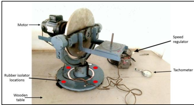
Fig. 1. Gyroscope coupled with varying speed motor experimental setup
