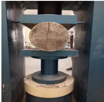
Figure 5: Testing of cylinder under CTM
