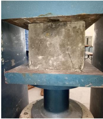
Figure 4: Testing of cube under CTM
