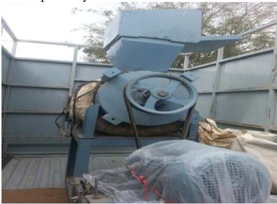
Fig: 1 Equipment Developed by M/S K K Plastic Waste Management Pvt Ltd. Bangalore, for processing Reclaimed Asphalt Pavement material.
