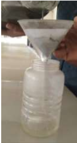
Fig. 1. Preparation of filtrate of cement slurry
