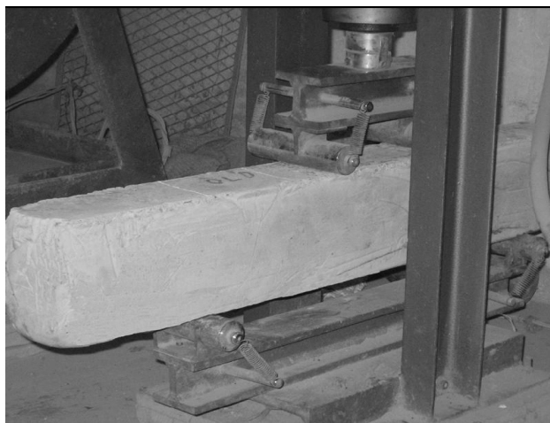
Fig6. Two point load test on reinforced concrete beam.
