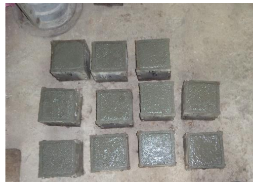
Figure 2: Cubes casted for Compression test
