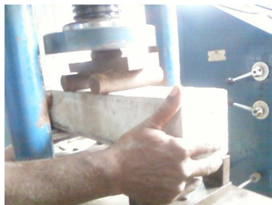
Figure 6: Flexural strength testing of a beam
