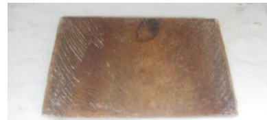
Figure 2.2.5 Treated coconut sheath composite plate
