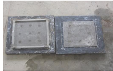
Figure 2.2.4 Compression moulding die
