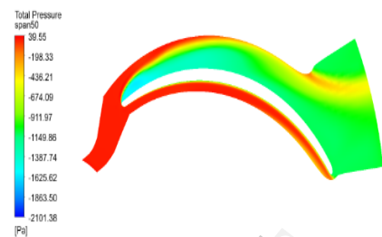
Fig12: Total Pressure 50% at 10000 rpm
