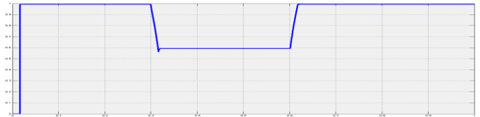
Figure 6. Load rms Voltage, short circuit in time 0.3 until 0.6 and without DVR
