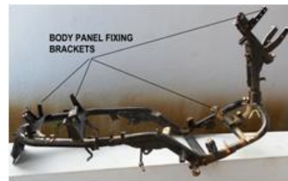
Figure2.1. Side view of the actual scooter chassis frame, mass=17Kg with extra body panel supporting brackets.
