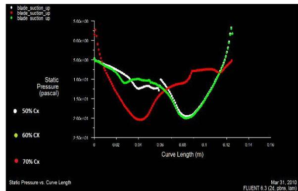
Graph 5.1 Static pressure Vs Curve length.
