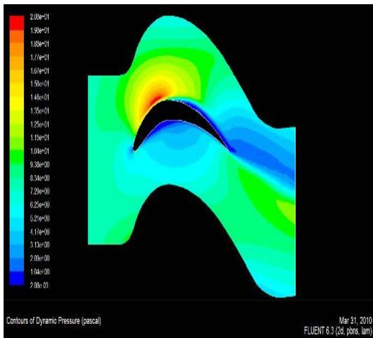
Fig-4c: Aerofoil with VG at its 50% Cx.
