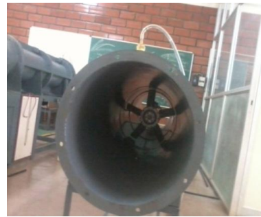
Fig.1. Ducted Axial fan test rig
