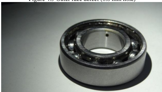
Figure 4.6 Outer race defect (0.8 mm hole)
