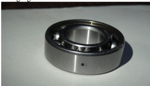
Figure 4.5 Outer race defect (0.8 mm hole)
