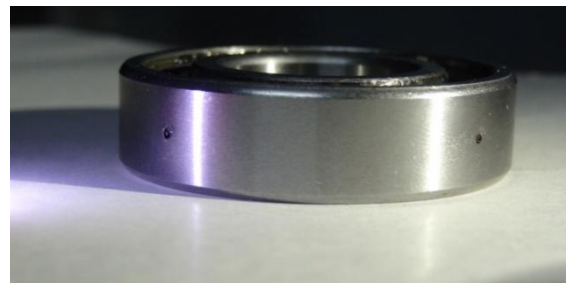
Figure 4.9 Two-outer race defects at 90 degree (0.8 mm holes)
