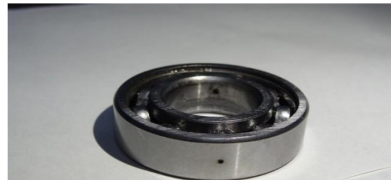
Figure 4.8 Inner-outer defects (0.8 mm holes)
