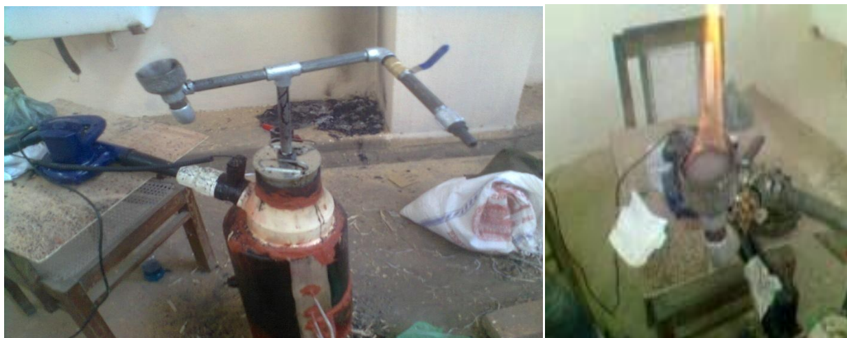
Figure 3.2: Experimental setup and burning flame in the burner.
