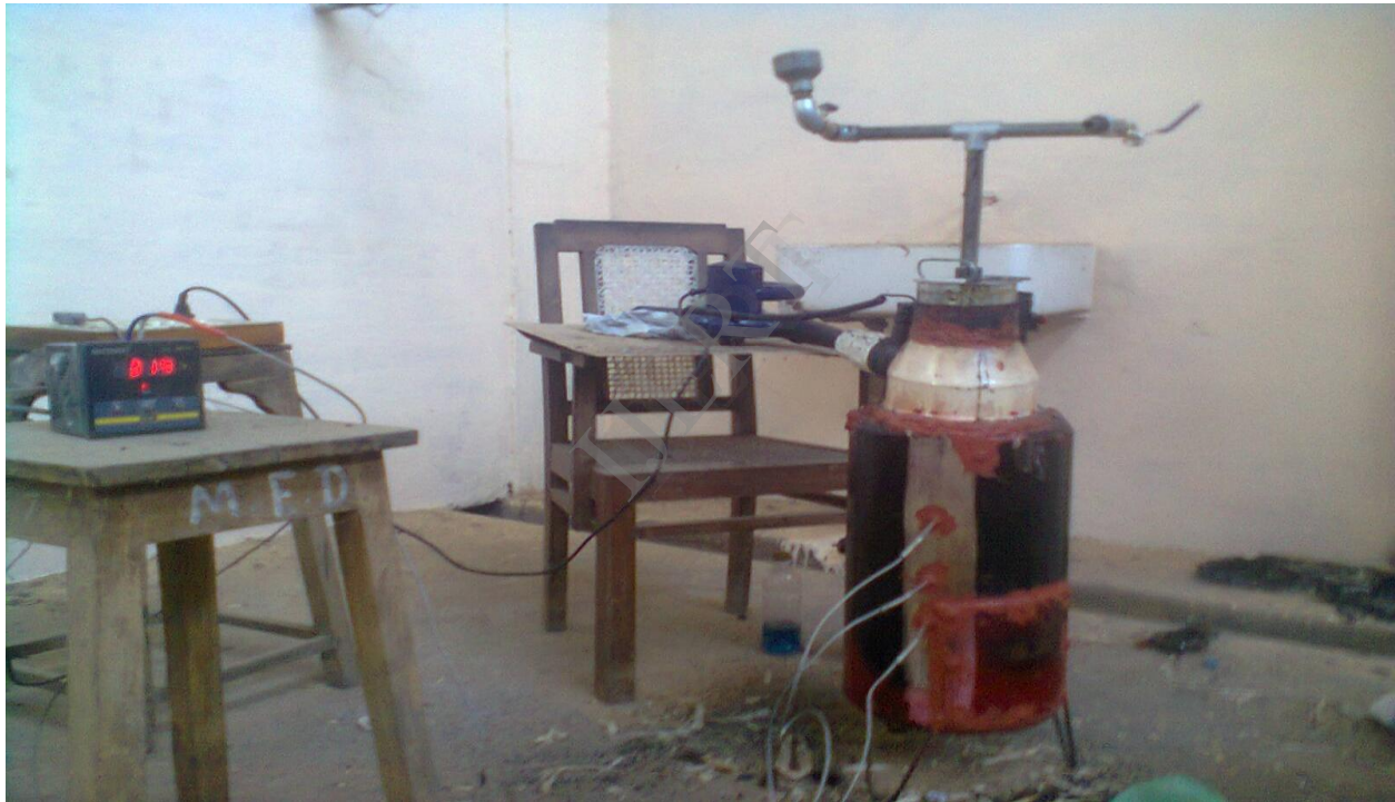
Figure 3.1 Experimental setup of updraft biomass gasifier
