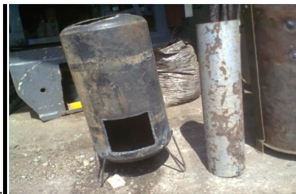
Figure 2.3 Cutting of the air tank
