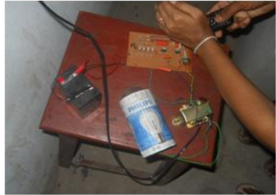
Figure 13: Control of lamp by LDR. When the light is falling on LDR, the lamp is going to be in OFF condition.
