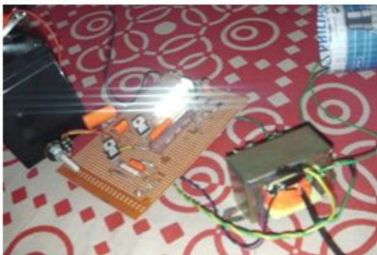
Figure 12: Emergency light is illuminated when no supply is
