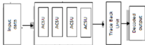
Fig. 3.6 Block diagram for proposed decoder
