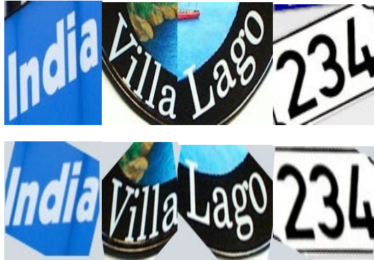
Fig.2. Result of orientation correction using proposed method. The first row shows sample images of oriented texts and the second row shows orientation correction using proposed method based on CNN.
