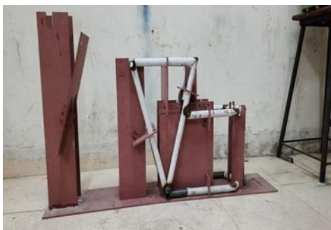
Fig 15. Fixtures for chassis manufacturing
