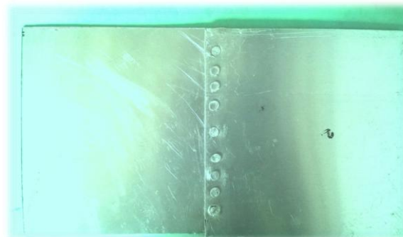
Fig 10 Aircraft skin single riveted joint in Aluminum alloy 2024 T3
