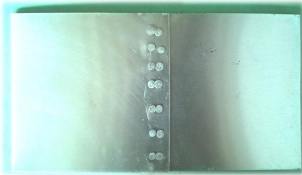
Fig 12 Aircraft skin double chain riveted joint in Aluminum alloy 2024 T3
