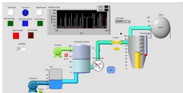
Fig. 5. Front Panel of Continuous monitoring system
