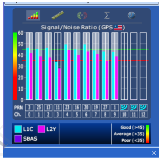
Figure 6. Satellite signal strength indicator window
