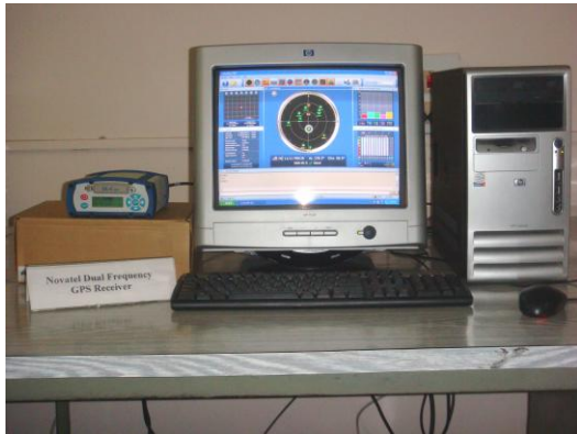
Figure 3. Data logging setup of DL-4plus GPS receiver
