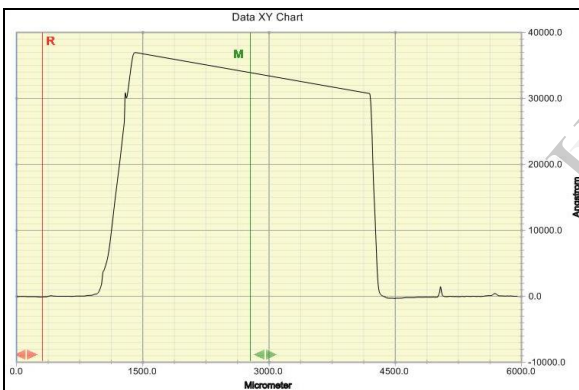
Fig. 12. Thin film of Aluminium on silicon wafer with thickness of 34,000Å°
