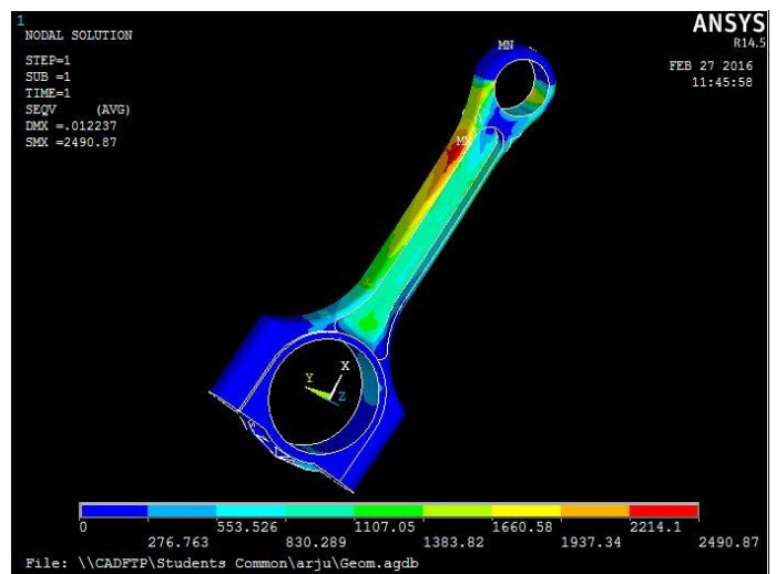
Fig.5: Von-Mises Stress of Steel
