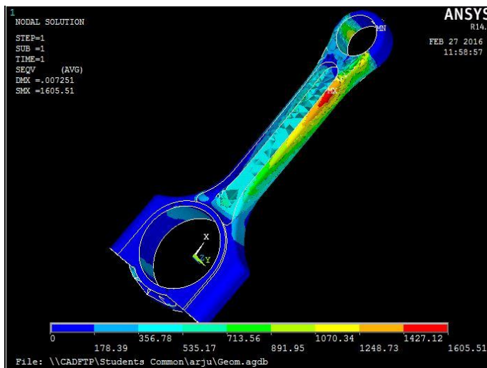
Fig.9: Von-Mises Stress of Steel
