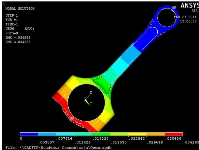
Fig.8: Total Deformation of Aluminium
