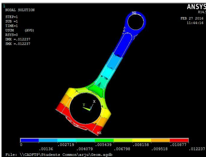
Fig.3: Total Deformation of Steel
