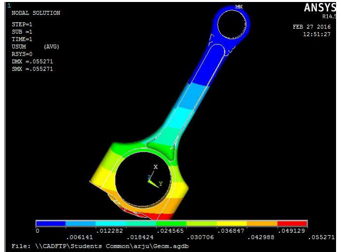
Fig.4: Total Deformation of Aluminium
