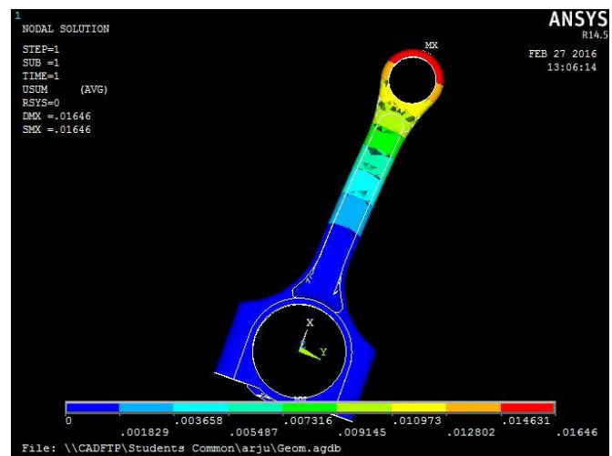
Fig.12: Total Deformation of Aluminium
