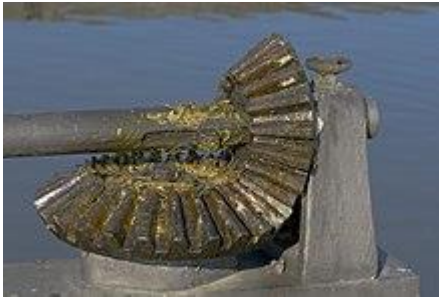
Fig 1.7 Bevel gear operating a lock gate
