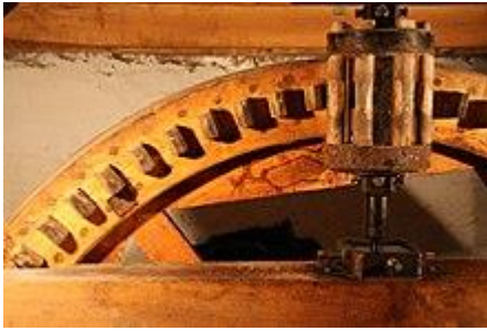
Fig 1.1 Wooden cogwheel driving a lantern pinion or cage gear
