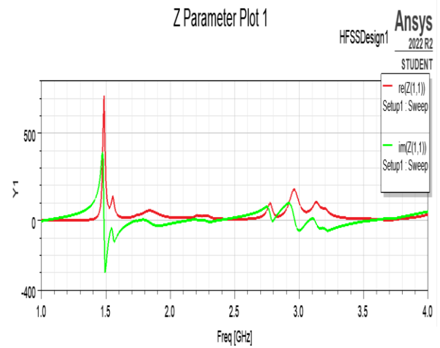
Fig. 3. U-slot microstrip patch antenna's simulated input impedance (with lump components)
