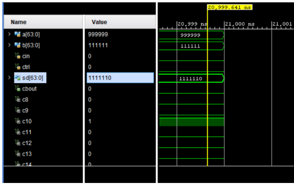
Fig.30 . Addition of 64 bit inputs A and B by existing design 1 RCA/ RBS.
