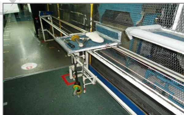
Figure 11* post implementation of the tools carrier
