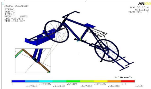
Figure 5: Load Case 1 (Von-Mises stresses)
