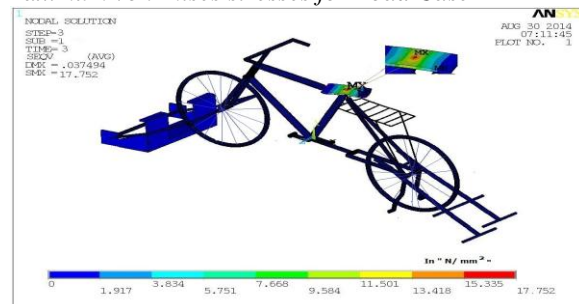
Figure 8: Load Case 2 (Von-Mises stresses)
