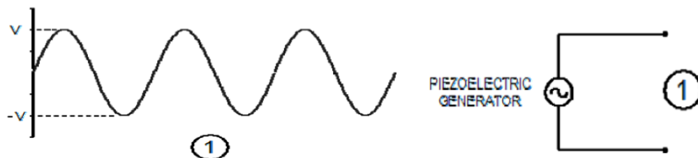
Figure5.1. Simple model of a piezoelectric generator
