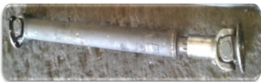
Figure-1: Universal Yoke Joint and Transmission Drive Shaft (Midi-712)
