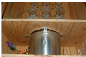
Figure 2. Fan positioned between the front panel and bulkhead
