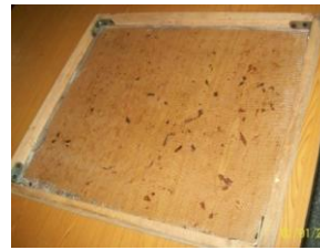
Figure 5. Wire mesh screen (1mm) laid over the finished tray frames
