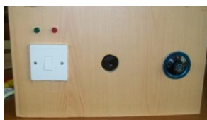
Figure 3. Air vent hole, switch and thermostat in the front panel
