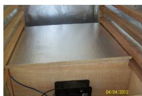
Figure 4. Heatshield in position over the heating chamber
