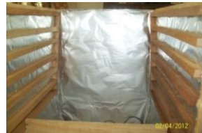
Figure 6. Tray place holders fixed to the walls of the dehydrator
