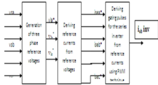
Fig. 6. Block diagram for generation of gating signals
