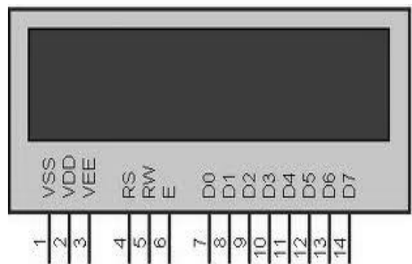
Fig.2: Schematic diagram of 16x2 LCD
