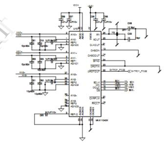
Here the system uses MAX11040K is 24 bits, four channels, simultaneous-sampling, sigmadelta analog-to-digital converters (ADCs) from MAXIM manufacturer. ADC s has four modulators simultaneously convert each fully differential analog input with a programmable data output rate ranging from 0.25ksps to 64ksps. The devices achieve 106dB SNR at 16ksps and 117dB. SNR at 1ksps (MAX11040K). The differential analog input range is  $\pm 2.2V$ .
