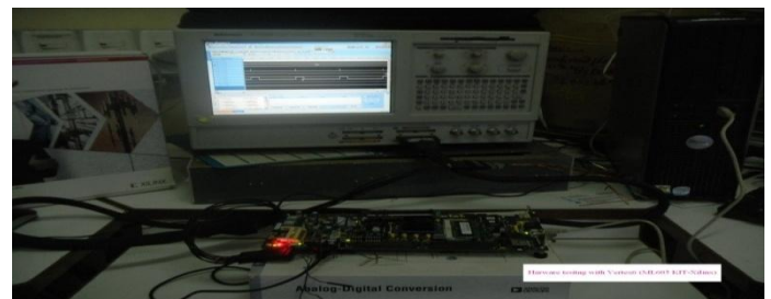
Fig.11 Testing with vertex 6 (ML605 kit) 1024-points IFFT/FFT with SNR=60 dB
