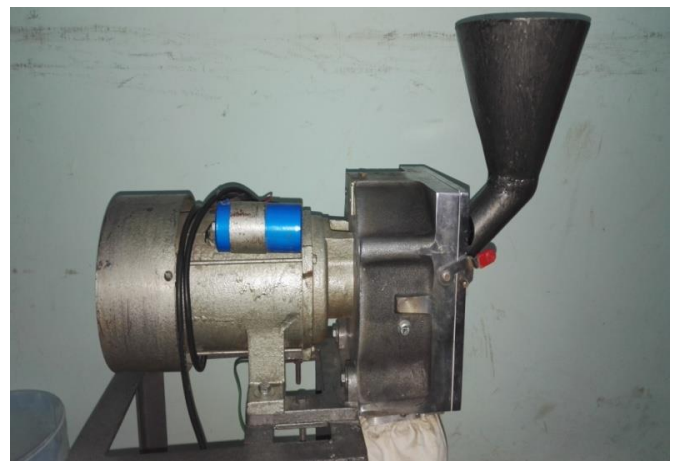
Figure 6:-Front View of Horizontal Impact Crusher
