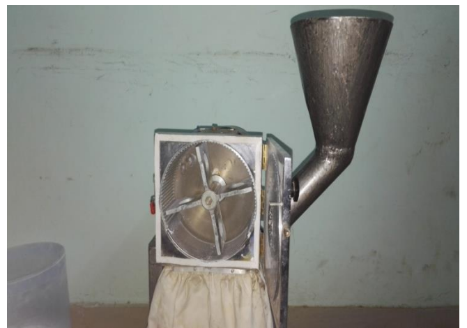
Figure 7:- SIDE VIEW OF Horizontal Impact Crusher
