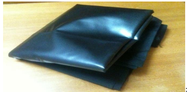
Fig 2.1 showing 1000D cordura nylon & PU coated
