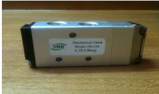
Fig 2.3. way normally closed push button operated spring return type
