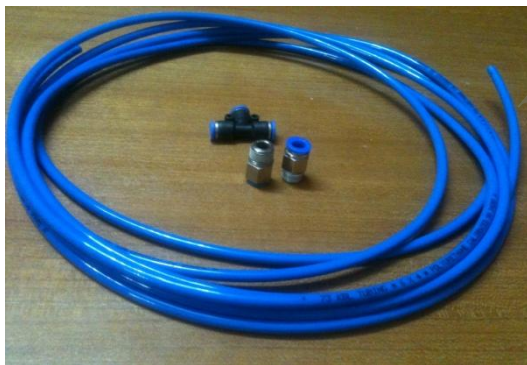
Fig 2.4: Hose pipe and 6mm one touch connector
