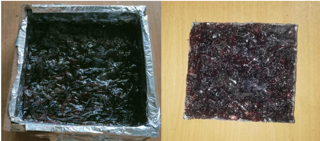
Fig4: Insulation Panel before Drying
