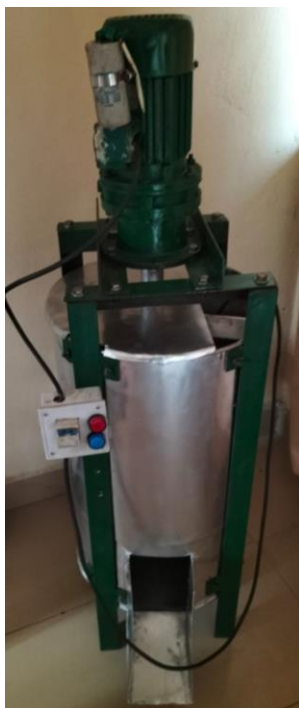
Fig 16: Locally fabricated Palm Fruit Digester
