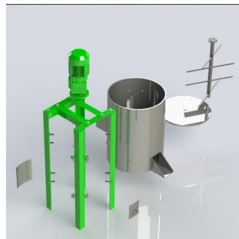
Fig 9: exploded view of palm fruit digester
