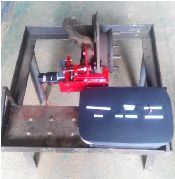
Figure 10 EMPB (complete system)
