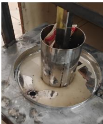
Figure 3. Millet milk extractor using lead actuator principle
