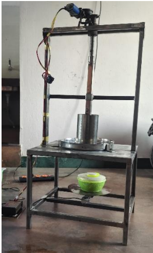
Figure 2. Front view of fabricated millet milk extractor using different components
