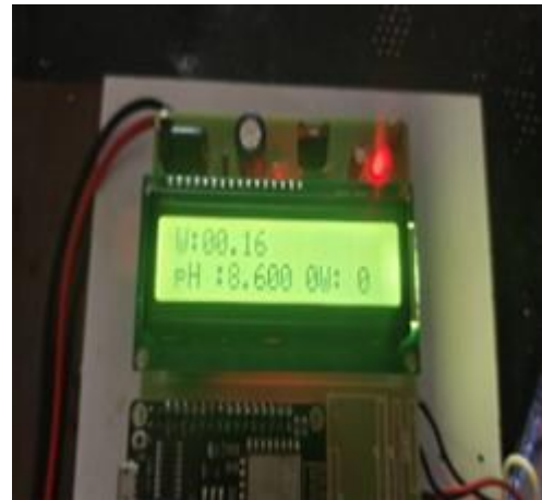
Figure 4. Sensors detecting quantity and pH of the extracted millet milk
