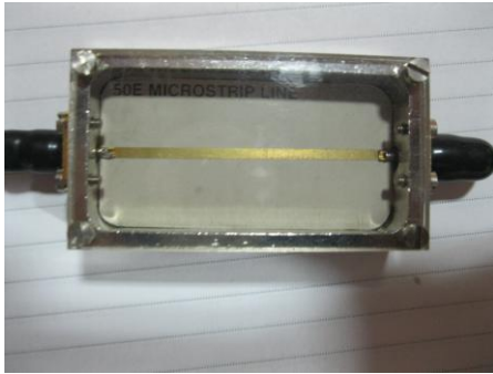
Fig. 2. Physical &amp; Constructional view of Microstrip lines
