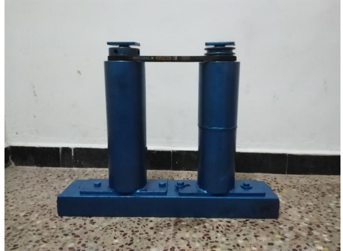
Fig.3. multi operated screw jack using belt drive
