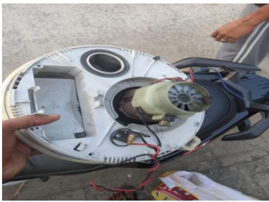
Fig 5. Motor used for suction
