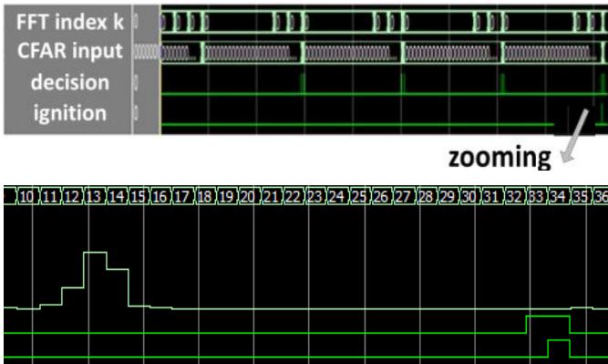
Fig. 18 Detailed Modelsim timing simulation in case of one moving target
