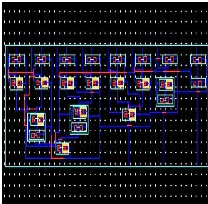
Fig. 23: Layout of thermometer to gray code converter.
