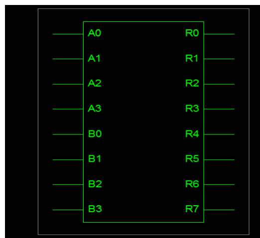
Fig 4 –RTL Schematic of 4×4 Vedic Multiplier
